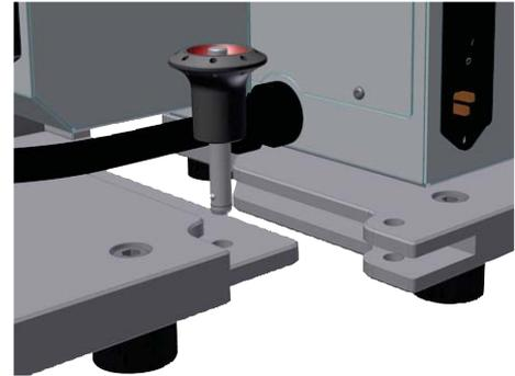
To conclude the preparations of the welding process, connect the two control cables: the one shown on the drawing to the right to the connector at the back of the mechanical structure and the one from the heating element to that on the right-hand side — when looking at the keypad — of the electronic control (see Sect. 3.2.2).
