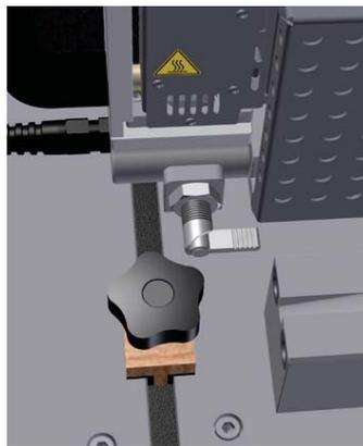
Star knob securing the base and tabletop plates, and transport lock (self-locking pin) of heating element
