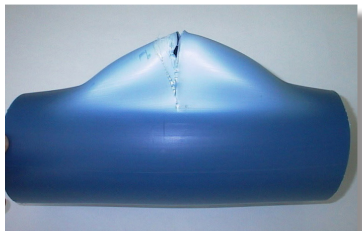
Air-Pro® over-pressurized ductile failure during burst test (pressure > 800psi)
