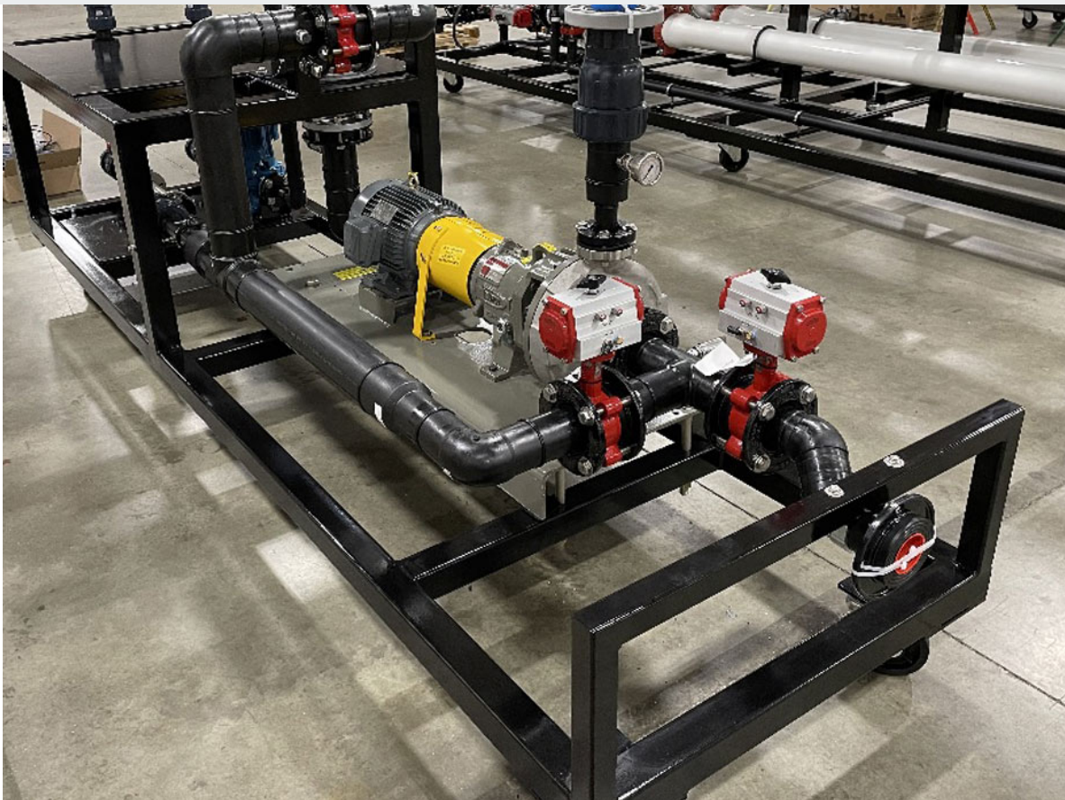
Picture 1: An example of yeast recovery skid assembled by Asahi/America, Inc. with HDPE pipe spools. The skid is installed in a brewery in the northeast U.S.
