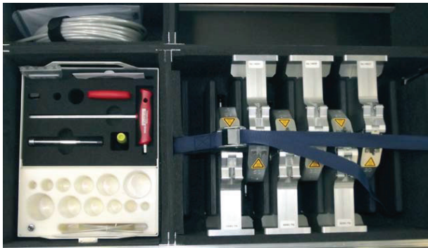
Box for tools and small parts (left, with a lid when shipping) and slots for heating element secured with a strap with buckle
