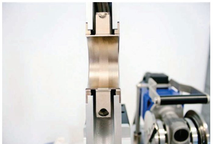
22 When done cleaning, touch "Ok" on the cleaning screen and close the heating element to let it cool down.
