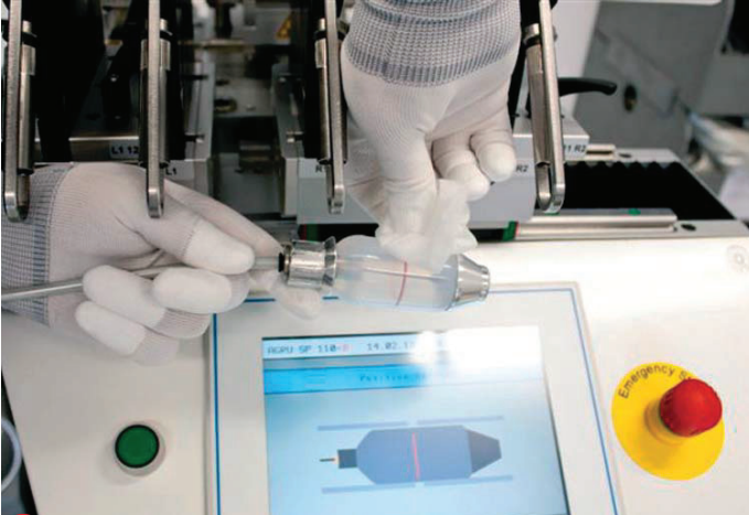
13 After facing and component alignment check, insert the inside balloon (see figures no. 26 - 30 depicting ...
