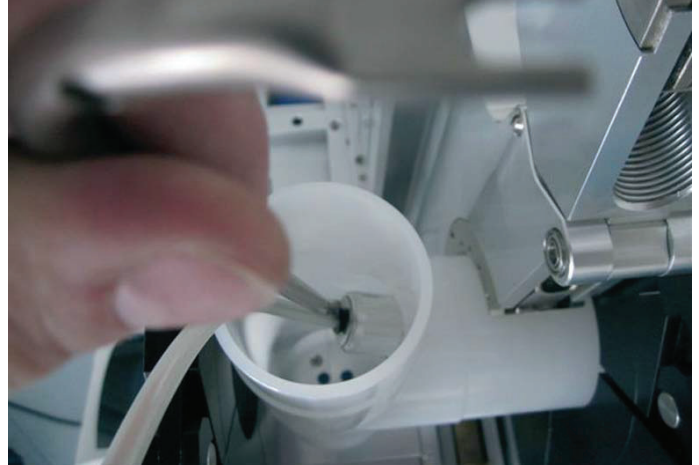
38 Remove the balloon from inside using the specialty tool.
