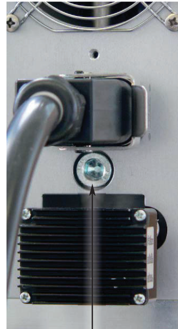
Screw for Locking the Heating Element
