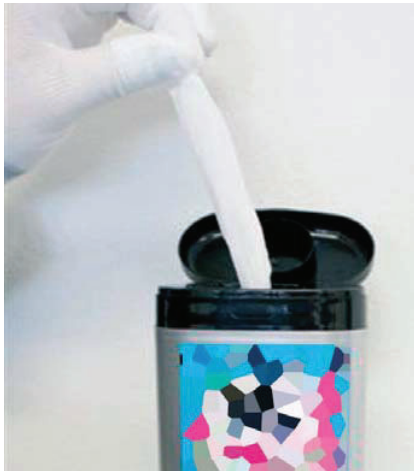
1 Wet a fibre-/lintless towel with isopropylic alcohol (ethanol content 70 - 80 %).
