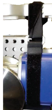
Strap with buckle and Velcro fastener to secure the handle of the facing tool
