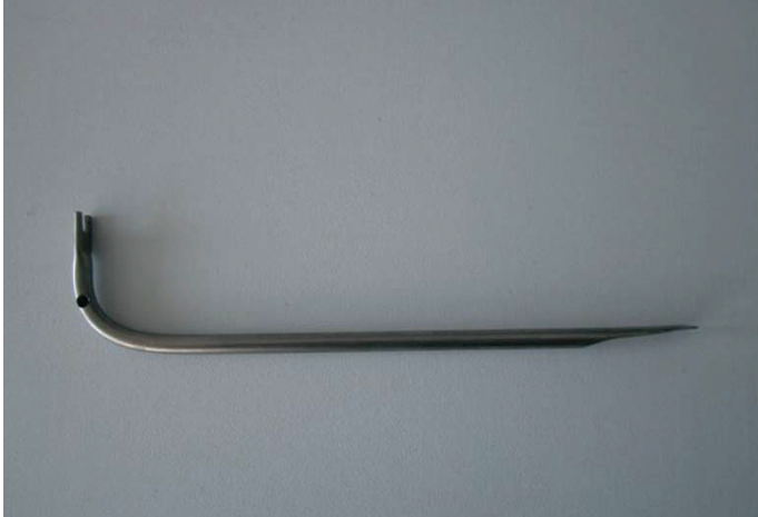
37 Specialty tool for removing the inside balloon from inside the new joint
