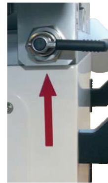
Transport lock of facing tool/heating element console; to lock/unlock it, pull out lever and turn it by 180 degrees
