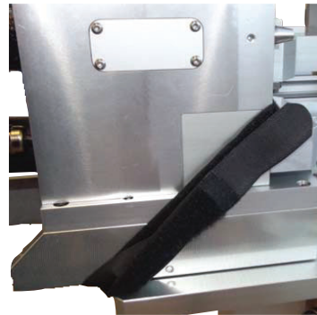
Strap with Velcro fastener to secure the base of the heating element support on the carriage
