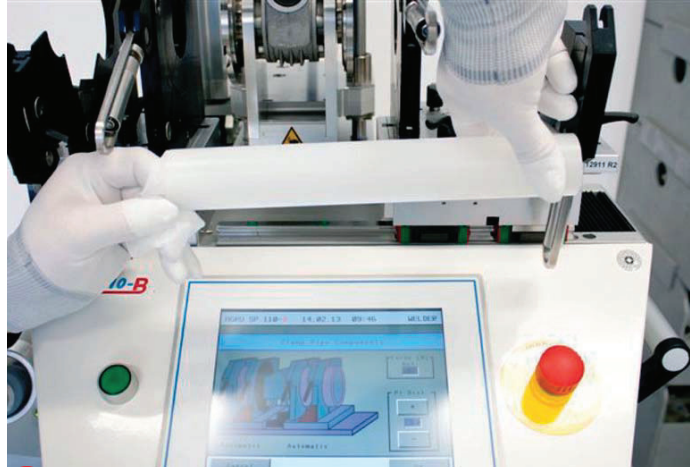
8 ... depicting the welding process); then clean butts of pipe ...
