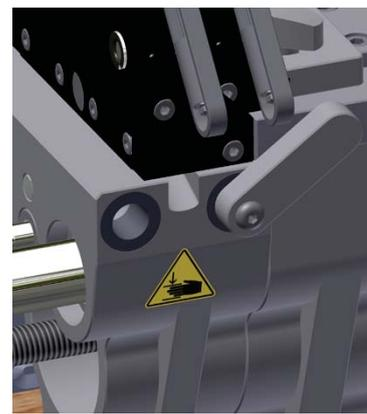
Transport lock of facing tool/heating element carrier and movable carriage (locking ball pin on the back to unlock locking bar)
