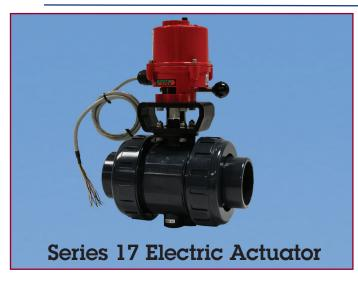
The Series 17 electric actuator features a reversing motor with multi-voltage capabilities; 85vac-265vac (50/60Hz), 24vdc. An internal heater, auxiliary switches, and two position indicating LED's, are standard equipment. Additional features include a permanently lubricated steel gear train, NEMA Type 4 & 6 enclosure with a thermally bonded powder coat finish, declutchable manual override, visual mechanical position indication, ISO bolt circle, and flying leads.
