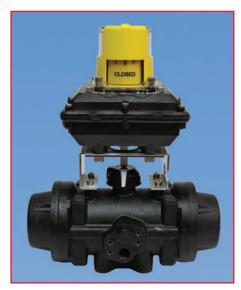
A limit switch box is mounted on and coupled to the actuator in order to operate position-indicating lights on control panels, to control other equipment such as pumps, compressors and mixers, to sequence other valves, or for feedback and PLC position confirmation. Two single pole, double throw (SPDT) switches are mounted in one enclosure and are activated by individual, adjustable cams.
